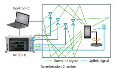
Moreover, it also supports the increasing number of test conditions demanded by higher antenna counts in UE units supporting LTE-Advanced CA and MIMO standards. Last, the shorter test time resulting from stable call processing performance is a key advantage of the MT8821C in various OTA test systems.
